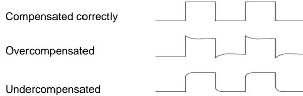
3. If necessary, use a nonmetallic screwdriver to adjust the variable capacity of your probe until the shape of the waveform turns to be the same as the above figure. Repeat this step as necessary. See the figure below for the way of adjustment.
