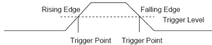
**Trigger Source:** Select the trigger source signal to CH1 or CH2. You can use the trigger source options to select the signal that the oscilloscope uses as a trigger.
